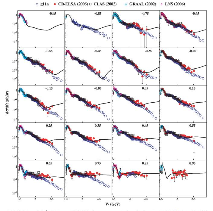
FIG. 10. (Color online)  $\frac{d\sigma}{d\Omega}(\mu b/sr)$  versus W (GeV) for the  $\gamma p \rightarrow p\eta$  reaction, in  $\cos \theta_{c.m.}^{\eta}$  bins, from CB-ELSA [2] (red solid circles), previous CLAS data [1] (open squares), GRAAL [3] (light-blue open triangles), LNS [4] (purple open diamonds), and this work (blue open circles). The centroid of each bin in  $\cos \theta_{c.m.}^{\eta}$  is labeled on each plot. The solid line is a SAID [17] fit to the earlier data.
