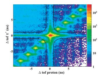
FIG. 2. (Color online)  $\Delta tof_{\pi^+}$  (ns) versus  $\Delta tof_p$  (ns): Particleidentification cut for a sample of events that pass a 10% confidencelevel cut when kinematically fit to the hypothesis  $\gamma p \rightarrow p\pi^+\pi^-(\pi^0)$ . The black lines indicate the timing cuts. Note the logarithmic scale on the intensity axis.
